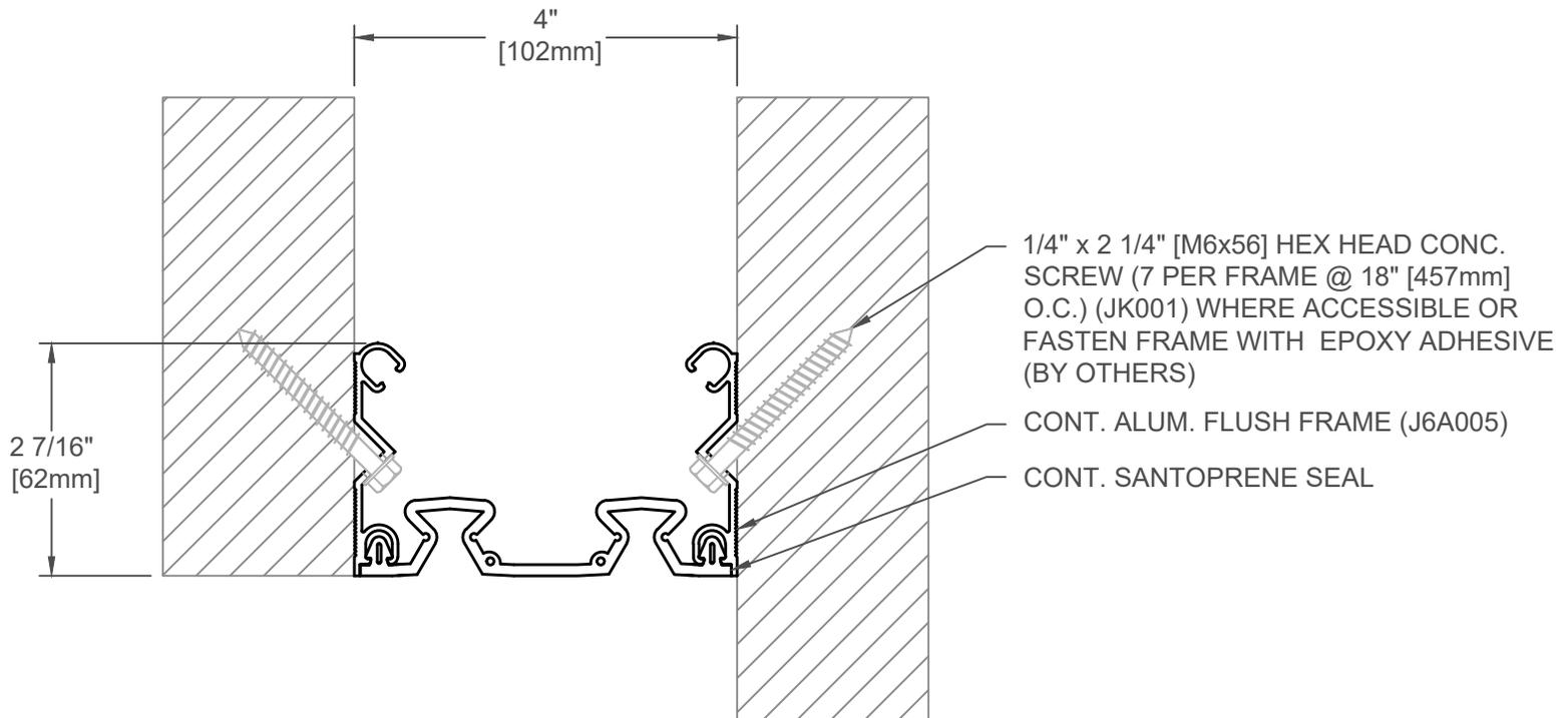
1/4" x 2 1/4" [M6x56] HEX HEAD CONC. SCREW (7 PER FRAME @ 18" [457mm] O.C.) (JK001) WHERE ACCESSIBLE OR FASTEN FRAME WITH EPOXY ADHESIVE (BY OTHERS)
