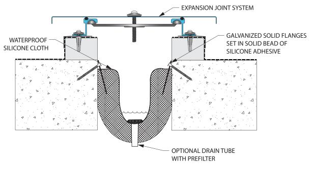
\*NOTE: Rated substrate hourly rating must not exceed the hourly rating of the F520 blanket assembly. Construction of the rated substrate is by others.
