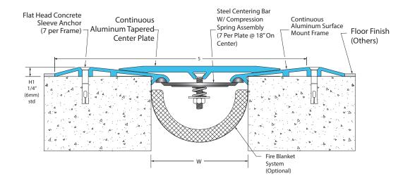
461-A01 Floor/Floor - New to Existing (4" (100mm) system shown)
