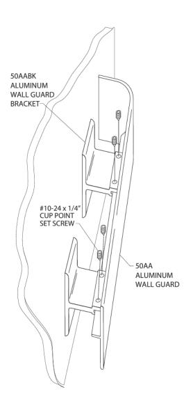
3. Position wall guard into mounting brackets. Tighten the wall guard into the brackets with set screws.
