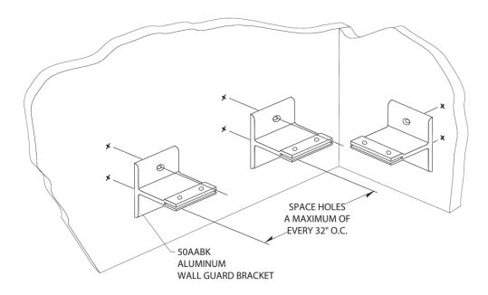
2. Drill marked holes with 19mm drill bit for toggle bolts (drywall installation) or 13mm drill bit for lead anchor (concrete wall installation). Mount brackets to wall, tighten screws to secure.
