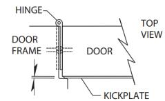
IF CLEARANCE ALLOWS KICKPLATE CAN BE FULL WIDTH OF DOOR
