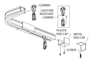
2. Slide the carriers on the track and attach end caps (plastic or metal) on the open ends. SEE FIG. 5
