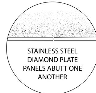
6. Repeat steps 2-5 to continue installation along entire length of the layout/wall, over laying the flat edge of each panel over the recessed flange of the one installed next to it. Ensure the top edge of each panel is flush and continuous with the panel next to it.
