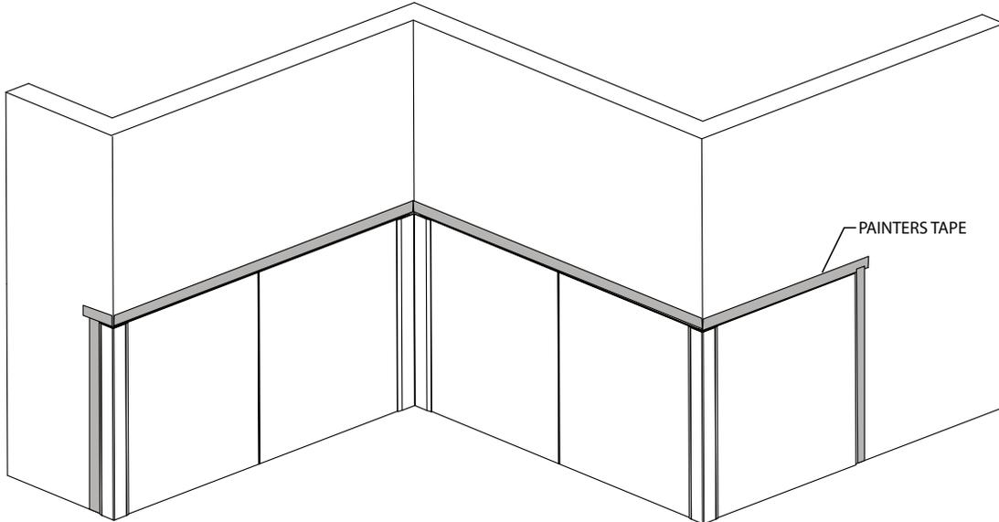
11. Apply a bead of color matched caulk to any exposed edge on the installation. Ensure the caulk penetrates into the gap between the panel and wall. After an edge has been sealed, use a plastic putty knife to scrape any excess sealant off of the panel face, then carefully remove the blue painters tape from the entire edge, by pulling back and away. Repeat for all exposed edges.
