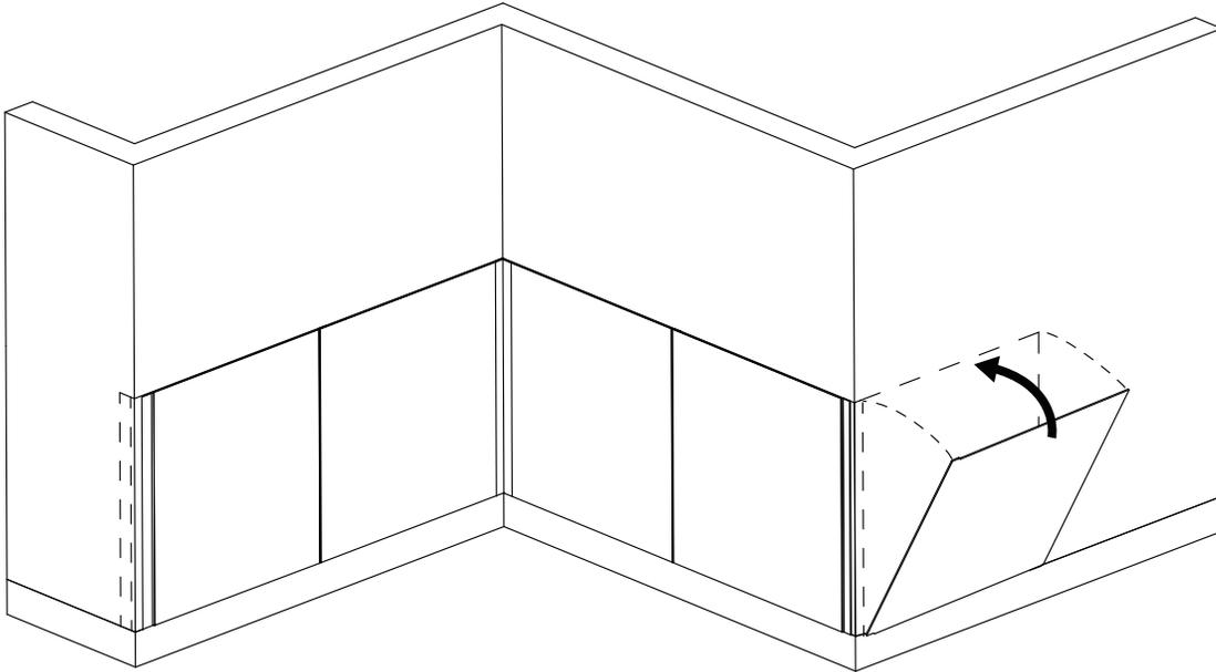
8. For corner trims, apply a single strip of foam tape to one of the backsides of the corner trim wings, then apply two (2) 1/4" [6mm] beads of PL-Premium® on back of the opposing wing. Position trim piece close to the corner, adhere the wing with the PL-Premium® to the panel first, then slide the trim piece into the corner so the wing with foam tape sets squarely into the corner; press the trim piece into the corner so the tape firmly against the panel to ensure adhesion.
